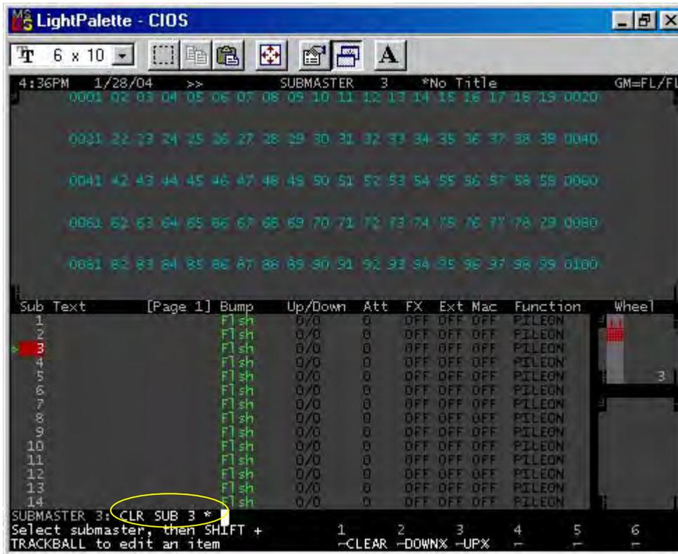
Now that sub 3 is cleared, you can add the correct channel in quickly and easily.
