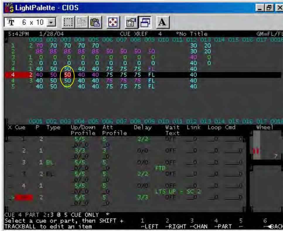
Channel 3 changed in cue 4 part 2 but now we have a “down” level for channel 3 in cue 5 so it is no longer a tracking level.
