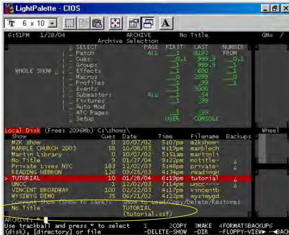
Note: Notice that the bottom of the screen shows you the Current Show (bottom left) and the Show to Load/Copy/Delete/Restore: (bottom right)
